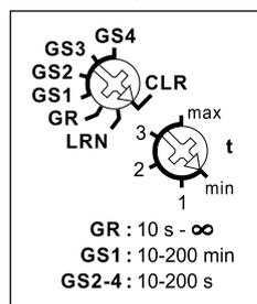
**With the top rotary switch** in the setting LRN up to 35 wireless pushbuttons can be assigned therefrom one or more central pushbuttons. The required function of this impulse group switch can then be selected:
