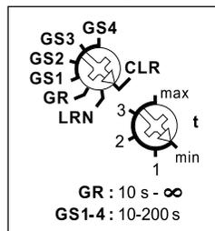
**With the top rotary switch** in the setting LRN up to 35 wireless pushbuttons can be assigned therefrom one or more central pushbuttons. The required function of this impulse group switch can then be selected:
