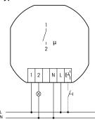
During teach-in, the function of the contact in quiescent position is defined as NO or NC. Closes the contact with at least one open window; it can then activate extraction hoods etc. or generate an alarm.
