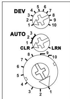
The own device address is set using the upper rotary switch.
