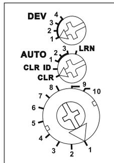
**Use the top rotary switch** to select the device address 1, 2, 3 or 4 of the addressed output FPV when the sensors are taught-in. Set the home device address in operation.
