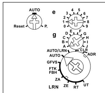
The **left rotary switch** is set to AUTO during operation.
