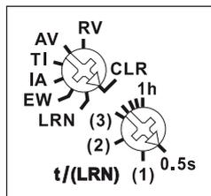
With the top rotary switch in the setting LRN up to 35 wireless pushbuttons can be assigned therefrom one or more central control pushbuttons. In addition, wireless window/door contacts (FTK) may have a NO or NC function when the window is open. If a direction switch is taught-in, a function (e.g. TI) can be started using the top switch (START) and stopped with the bottom switch (STOP). The required function of the wireless actuator can then be selected:
