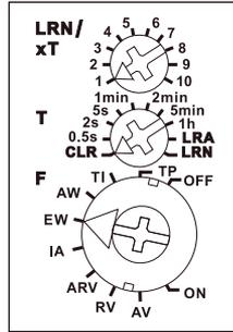
Teach-in takes place **using the top and middle rotary switches** and then the time is set. T is the time base and xT the multiplier.
