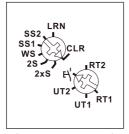
With the top rotary switch in the setting LRN up to 35 wireless pushbuttons can be assigned therefrom one ore more central control pushbuttons. The required function of this multifunction impulse switch can then be selected. Switching will be visualised by flashing of the LED.
