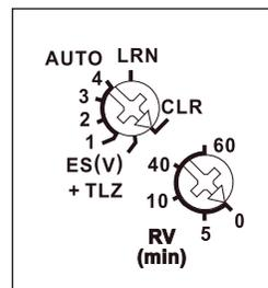
**With the top rotary switch** in the setting LRN up to 35 wireless pushbuttons can be assigned therefrom one or more central control pushbuttons. In addition, wireless motion and brightness sensors. Then select the required operating mode:
