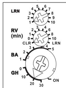
The upper rotary switch LRN is required for teach-in and for setting the base brightness.
