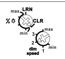
The flashing of the LED as soon as a new setting range has been reached when turning the rotary switch helps to find the desired position reliably.
