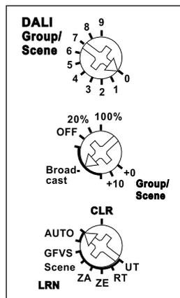
**Operation:** After switching on the power supply, the complete DALI bus is scanned and the red LED on the FDG71L flickers for several seconds. All DALI devices present will be recognized with their short address and following adjustments will be read: MIN Level, Dimmspeed (fade rate & fade time) and group affiliation. The least possible minimum brightness is determined from this data and the dimming speed for groups 0..15. All DALI devices in a group must have the
