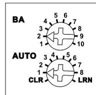
**The lower rotary switch** is required to teach in encrypted sensors and can be turned to AUTO 1 in operation.
