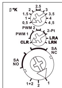
**Then set the operating mode using the middle rotary switch:** PWM 1 for valves with thermoelectric actuator, T = 4 minutes. PWM 2 for valves with motor-driven actuator, T = 15 minutes. 2-Pt for 2-point control.
