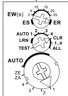
**The upper rotary switch** defines the function of the 4 channels together as impulse switch (ES), fleeting NO contact (EW) or relay (ER). In ES function, central control commands ON/OFF can be taught-in. In EW function, a wiping time of 2 to 25 seconds can be set.
