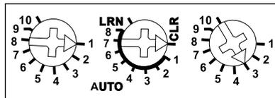
The middle rotary switch must be set to position LRN for teach-in. Set the required operating mode when the fan actuator is in operation.
