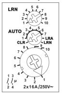
**The middle rotary switch** must be set to position LRN for teach-in. Set the required operating mode when the fan actuator is in operation.
