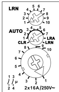
**The middle rotary switch** must be set to position LRN for teach-in. Set the required operating mode when the fan actuator is in operation.
