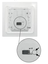
Insert the encryption plug and operate the rocker.
