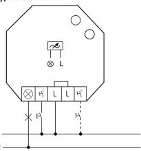
Control by pushbutton switches or lightswitch.
