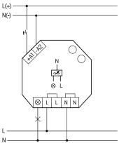
Universal control voltage 8..230 V UC, supply voltage and switching voltage 230 V ~ 50/60Hz
