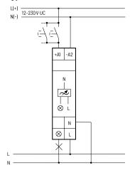
Supply and switching voltage 230 V ~ 50/60Hz
