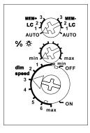
shows control commands. It starts blinking after 15 seconds if a pushbutton is inhibited. If the **MEM+** setting range is selected, the memory function is active and the last brightness level set is saved when the device is switched off. If the setting range **MEM-** is selected, the **memory function** is switched off and it is always switched on with maximum brightness. Dimmable energy-saving lamps must be operated on AUTO and MEM-.
