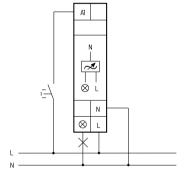
Supply- and switching voltage 110-240 V ~ 50/60Hz
