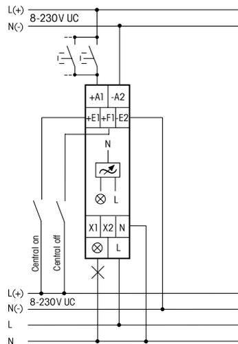
**Function 'DSD'** = Same as universal dimmer switch EUD but also comprising activation via two direction switches on the universal voltage control inputs 8..230V UC.
