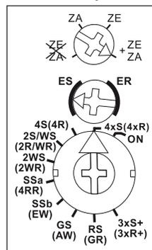
With the upper rotary switch this impulse switch with integrated relay function can be partly or completely excluded from central control:
