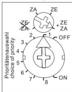
With the upper rotary switch this impulse switch can be partly or completely excluded from central control:
