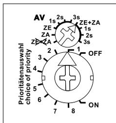
**With the upper rotary switch** this impulse switch can be partly or completely excluded from central control:
