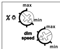
**With the top rotary switch** %⚙️ the minimum brightness level (completely dimmed down) can be adjusted.
