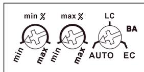
Minimum brightness (fully dimmed down) is adjustable **using the left % rotary switch.**
