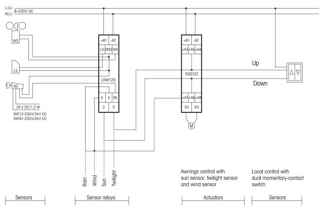
When controlling with 230 V (+B1= L, -A2=N) the 230 V awning motor is directly connected to K2, K3 and N. Otherwise a motor isolating relay MTR12-UC must be interconnected to K2/K3.
