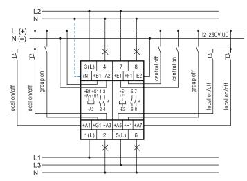
If N is connected, the zero passage switching is active at the contacts 1-2, 3-4 and 5-6.
