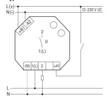
If N is connected, the zero passage switching is active.
