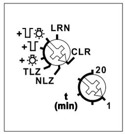
**With the top rotary switch** in the setting LRN up to 35 wireless pushbuttons and/or wireless motion/brightness sensors FBH can be assigned of which one or more central pushbuttons. The required function of this staircase off-delay timer can then be selected.
