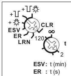
With the top rotary switch in the setting LRN up to 35 wireless pushbuttons can be assigned therefrom one ore more central control pushbuttons. In addition wireless window/door contacts with the function N/O contact or N/C contact while the window is open. The required function of the impulse switch with integrated relay function can then be selected:
