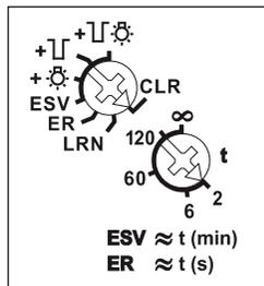
With the **top rotary switch** in the setting LRN up to 35 wireless pushbuttons can be assigned, of which one or more central control push-buttons. In addition wireless window/door contacts with the function N/O contact or N/C contact while the window is open.
